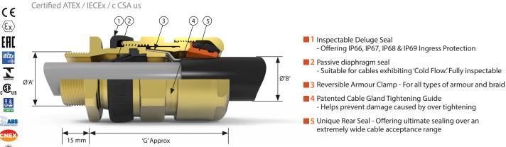
The 501/453 Universal Cable Gland is dual certified Exe/Exd, robust and for use with single wire armour 'W', wire braid 'X', steel tape armour 'Z', elastomer and plastic insulated cables. For particular use with cables that exhibit 'Cold Flow' characteristics. This cable gland is the first and only cable gland capable of being upgraded to a barrier type solution in the field. see below for more details. See technical section for installation rules and regulations.
