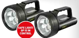
The advanced electronics prevent deep discharge of the battery and indicate low battery charge. Both Zone 0 and Zone 1 models are available with the The Atexor emergency function (EM) and blinking mode (BK). When the IL-800 hand lamp with EM-function is in ILC4 charger, it can detect a power outage and turn on automatically. When the remaining battery power is getting low, the beam stars to blink at 15 second intervals.
